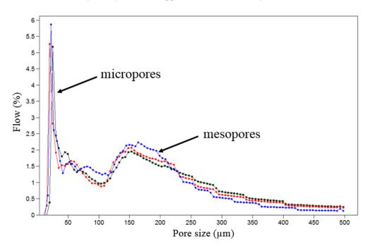
Figure 1: Through-thickness pore size distribution of three samples from a Signatex SC6227270 carbon fabric.
